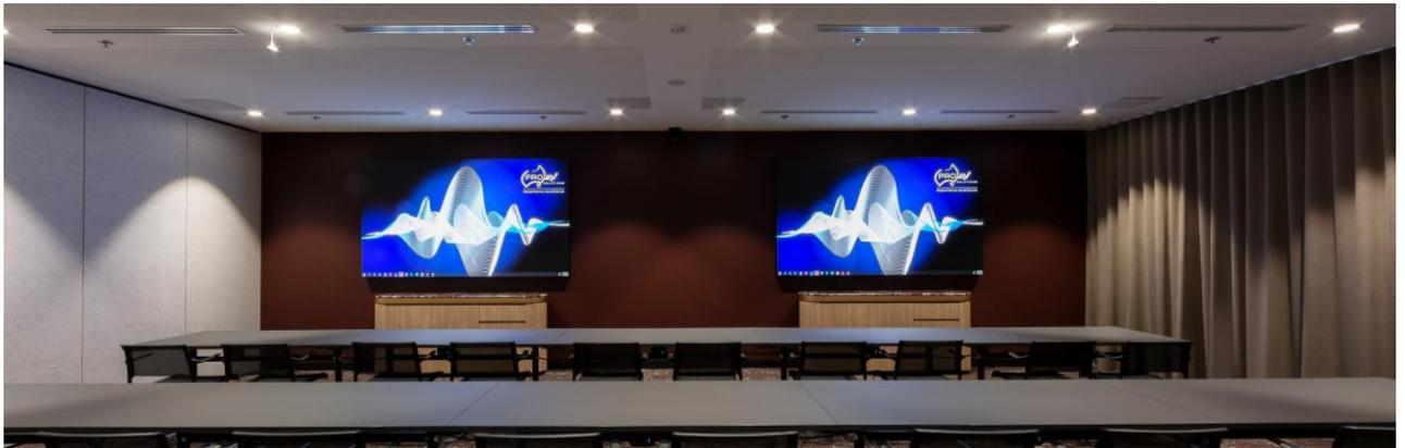
Two training rooms include one 110" The Wall, 4 Bose EdgeMax ceiling speakers for premium room-filling coverage, and Cisco Room Kit Quad cameras for the video conferencing system. The third is a double-size training room, comprising of two 110" Samsung The Wall, 8 Bose EdgeMax, 4 Ceiling Mics, and 2 PTZ Cameras located at front and back of the room and connected to a Cisco Codex SX80.
